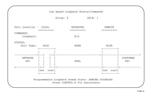
Figure 541-6a. HLXC Customer Loopback Screen
